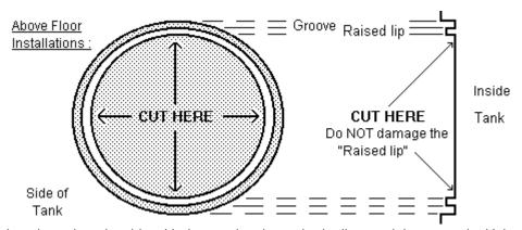
Lay the unit on its side with the previously marked toilet pan inlet upwards. Using a Stanley knife or jig saw, cut a circular hole through the tank at the point indicated by the arrows and "CUT HERE" sign. Be careful to cut at the INSIDE corner and NOT TO DAMAGE the inner raised lip for fitting the pan seal.
