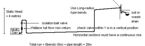
Plot the intersection of metres static head and metres total run on the chart below (Figure 5).
