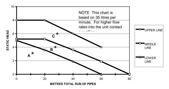
NB: The above chart and figures are based on using Class B or D or 4.5 PVC pressure pipes and one WALLACE 32 mm full flow non-clog non-return ball check valve. This will ensure a minimum delivery flow of 35 litres per minute from the WALLACE MULTI-SAN. This is in excess of the highest output domestic washing machine that is currently known to be available. If you are uncertain, call your appliance supplier for the output flow for your particular unit.
