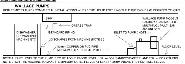
If not practical talk to Wallace Pumps about cold water solenoid valve injection systems for dishwasher discharge.
