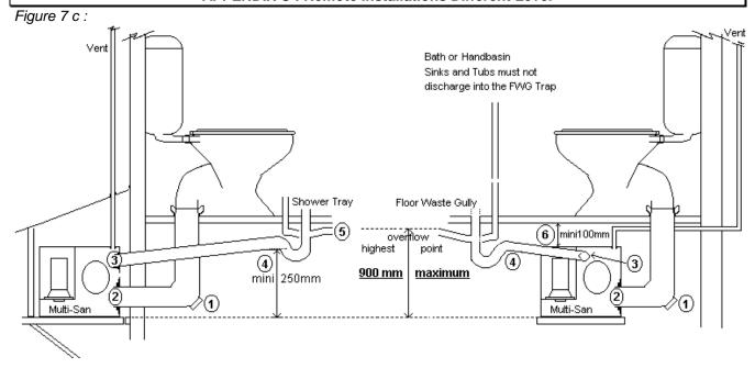
These remote installations must have the pan vented as normally required for a gravity flow installation, this vent is not shown on these diagrams.
